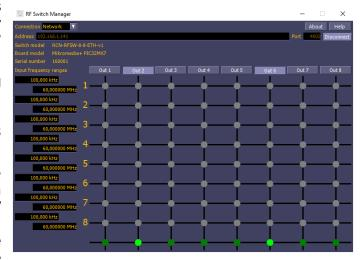
The frequency ranges for the 8 inputs can be customized based on the negotiated minimum requirements, considering also the available pre-built modules. There is an upper limit frequency of 3GHz due to the switching modules parameters.
